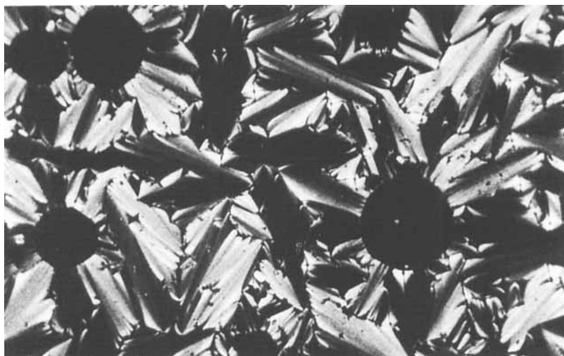
FIGURE 10a Photomicrographs for 4-propionyl-4'- n -heptanoyloxyazobenzene ( n = 5 ), crossed polarizers, magnification 80\times . S_4 phase.
